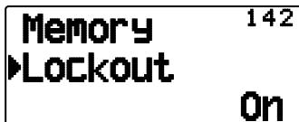
3 Set the lockout to "On" to lock the channel out of the scanning sequence.
